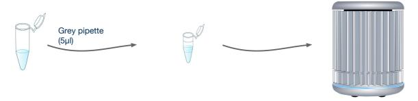
For each sample you wish to analyse, use the grey pipette to add 5µl of your RNA sample to the required reaction tubes. Close these tubes after adding the sample. Always change pipette tips between samples.
