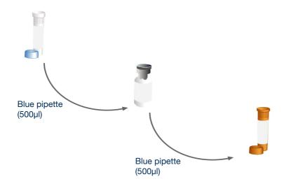
Use the blue pipette to transfer 500µl\* of the oasig Master Mix resuspension buffer into the tube of lyophilised oasig Master Mix and mix well by gently swirling. Then transfer all of that master mix into the brown tube labelled H.influenzae primers/probe.
