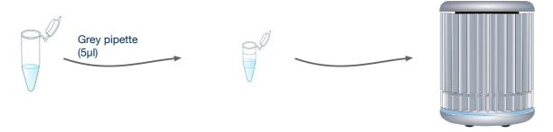
For each sample you wish to analyse, use the grey pipette to add 5µl of your RNA sample to the required reaction tubes. Close these tubes after adding the sample. Always change pipette tips between samples.
