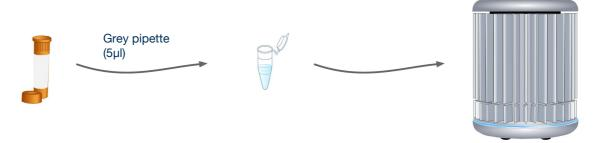
For every reaction to be run, use the grey pipette to add 5µl of your JEV primers/probe mix to every tube.
