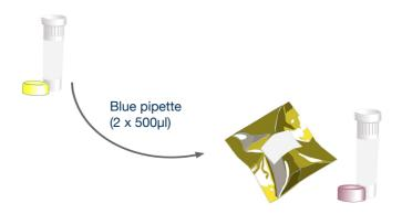
Use the blue pipette to transfer  $1000\mu l$  (2 x  $500\mu l$ ) of template preparation buffer into the positive control template tube. Cap and shake tube to mix.
