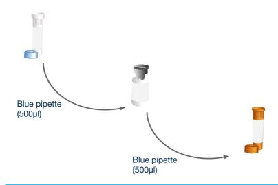
Use the blue pipette to transfer 500µl\* of the oasig Master Mix resuspension buffer into the tube of lyophilised oasig Master Mix and mix well by gently swirling. Then transfer all of that master mix into the brown tube labelled L.intracellularis primers/probe.
