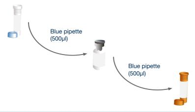
Use the blue pipette to transfer 500µl\* of the oasig Master Mix resuspension buffer into the tube of lyophilised oasig Master Mix and mix well by gently swirling. Then transfer all of that master mix into the brown tube labelled Whiting primers/probe.
