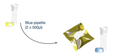
Use the blue pipette to transfer  $1000\mu$ I (2 x  $500\mu$ I) of template preparation buffer into the Internal Extraction Control DNA tube. Cap and shake tube to mix.
