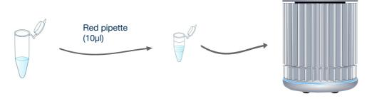
For each sample you wish to analyse, use the red pipette to add  $10\mu$ l of your DNA sample to the required reaction tubes. Close these tubes after adding the sample. Always change pipette tips between samples.
