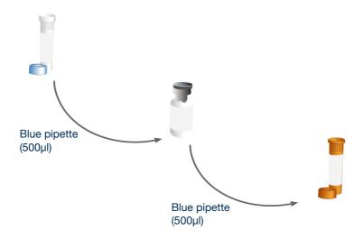
Use the blue pipette to transfer 500µl\* of the oasig Master Mix resuspension buffer into the tube of lyophilised oasig Master Mix and mix well by gently swirling. Then transfer all of that master mix into the brown tube labelled Sheep primers/probe.
