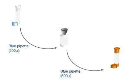
Use the blue pipette to transfer 500µl\* of the oasig Master Mix resuspension buffer into the tube of lyophilised oasig Master Mix and mix well by gently swirling. Then transfer all of that master mix into the brown tube labelled P.falciparum primers/probe.
