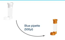
Then use the blue pipette to transfer 500µl of water into the brown tube labelled PPRV primers/probe. Cap and shake tube to mix. A thorough shake is essential to ensure that all components are resuspended. Failure to mix well can produce poor kit performance.
