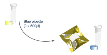
Use the blue pipette to transfer  $1000\mu$ I (2 x  $500\mu$ I) of template preparation buffer into the Internal Extraction Control DNA tube. Cap and shake tube to mix.
