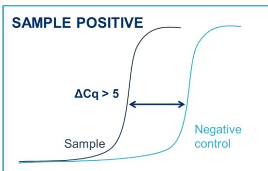
If the sample amplifies > 5 Cq earlier than the negative control, then the sample should be reinterpreted (via the table above) with the negative control verified as negative.
