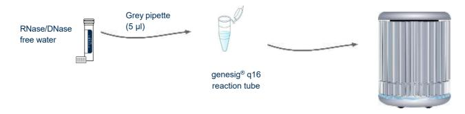
For each test you will require a negative control. Instead of RNA, water is used. The negative control sample should give a negative test result and thereby prove that any positive samples really are positive, and not tested positive due to contamination.
