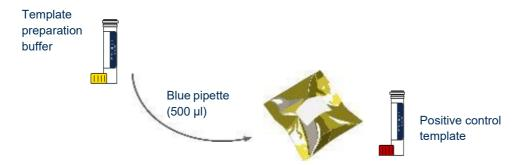
Use the blue pipette to transfer  $500 \, \mu l$  of template preparation buffer into the positive control template tube. Cap and shake tube to mix.
