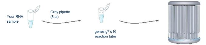
For each sample you wish to analyse, use the grey pipette to add 5 µl of your RNA sample to the required reaction tube (already containing primer/probe mix and oasig®PLUS OneStep Master Mix). Close these tubes after adding the sample. Always change pipette tips between samples.
