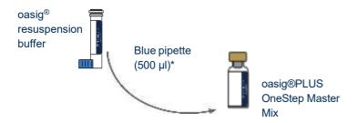
Use the blue pipette to transfer 500 µI\* of the oasig® resuspension buffer into the tube of oasig®PLUS OneStep Master Mix and mix well by gently swirling.
