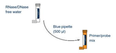
Then use the blue pipette to transfer 500 µl of water into the brown tube labelled Rabies v2.0 primer/probe mix. Cap and leave for 10 minutes to rehydrate. Then shake tube to mix. A thorough shake is essential to ensure that all components are resuspended. Failure to mix well can produce poor kit performance.
