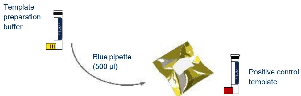
Use the blue pipette to transfer 500 µl of template preparation buffer into each of the positive control template tubes. Cap and shake each tube to mix.
