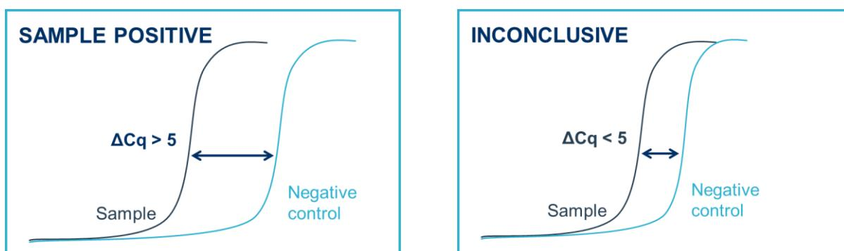
If the sample amplifies  $> 5$  Cq earlier than the negative control, then the sample should be reinterpreted (via the table above) with the negative control verified as negative.
