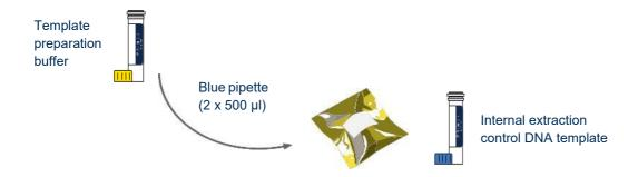
Use the blue pipette to transfer 1000  $\mu$ l (2 x 500  $\mu$ l) of template preparation buffer into the Internal Extraction Control DNA template tube. Cap and shake tube to mix.
