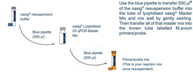
\*Transferring 525 µI of the oasig® resuspension buffer to your oasig® Lyophilised 2X qPCR Master Mix (instead of the 500 µI recommended above) will enable you to take full advantage of the 50 reactions by accounting for volume losses during pipetting. In order to do so with the genesig® Easy fixed volume pipettes use 1x blue, 2x red and 1x grey pipettes to make the total volume. Please be assured that this will not adversely affect the efficiency of the test.
