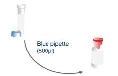
Use the blue pipette to transfer 500µl\* of the oasig OneStep Master Mix resuspension buffer into the tube of lyophilised oasig OneStep Master Mix and mix well by gently swirling.
