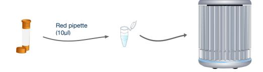
For every reaction to be run, use the red pipette to add 10µl of your T.forsythia reaction mix to every tube.
