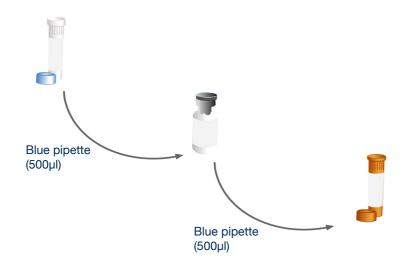
Use the blue pipette to transfer 500µl\* of the oasig Master Mix resuspension buffer into the tube of lyophilised oasig Master Mix and mix well by gently swirling. Then transfer all of that master mix into the brown tube labelled P.salmonis primers/probe.
