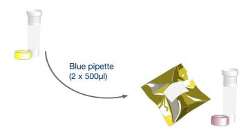
Use the blue pipette to transfer  $1000\mu$ I (2 x  $500\mu$ I) of template preparation buffer into the positive control template tube. Cap and shake tube to mix.
