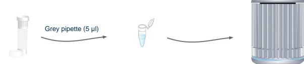
For each test, you will require a negative control. Instead of RNA, water is used. This sample should typically prove negative, thus proving that all of your positive samples are positive.
