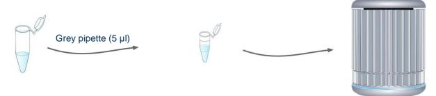
For each sample, you wish to analyse, use the grey pipette to add 5  $\mu$ I of your RNA sample to the required reaction tubes. Close these tubes after adding the sample. Always change pipette tips between samples.
