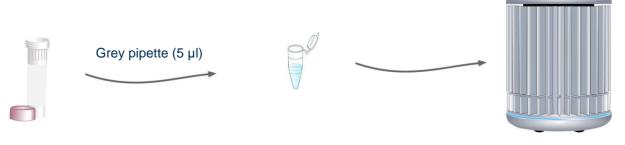
Take great care when setting up your positive control. The positive control template has the potential to give you a false positive signal in your other samples. Set up the positive controls last after all other sample tubes are closed. Always change pipette tips between samples. You may even choose to set up positive controls in a separate room.
