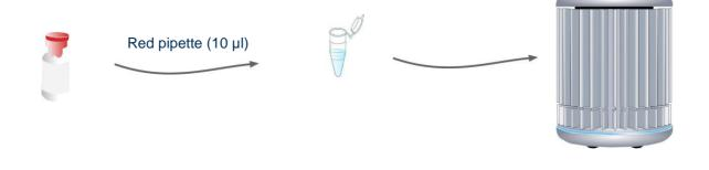
For every reaction run, use the red pipette to add 10 µl of the oasig<sup>™</sup> OneStep Master Mix to the tubes containing primer/probe mix.
