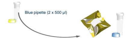
Use the blue pipette to transfer 1000  $\mu$ I (2 x 500  $\mu$ I) of template preparation buffer into the Internal Extraction Control RNA tube. Cap and shake tube to mix.
