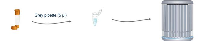
For every reaction run, use the grey pipette to add 5 µl of your H5N1 primers/probe mix to every tube.
