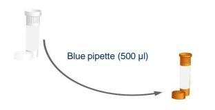
Then use the blue pipette to transfer 500  $\mu$ l of water into the brown tube labelled H5 or N1 primers/probe. Cap and shake tube to mix. A thorough shake is essential to ensure that all components are resuspended. Failure to mix well can produce poor kit performance.
