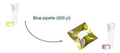
Use the blue pipette to transfer 500  $\mu$ I of template preparation buffer into the positive control template tube. Cap and shake tube to mix.
