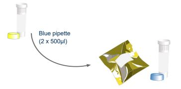
Use the blue pipette to transfer  $1000\mu$ l (2 x  $500\mu$ l) of template preparation buffer into the Internal Extraction Control DNA tube. Cap and shake tube to mix.
