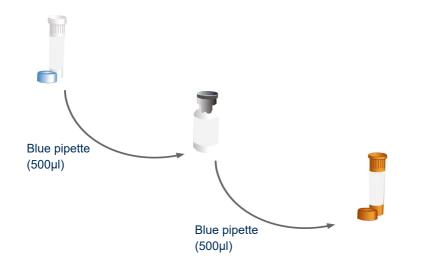
Use the blue pipette to transfer 500µl\* of the oasig Master Mix resuspension buffer into the tube of lyophilised oasig Master Mix and mix well by gently swirling. Then transfer all of that master mix into the brown tube labelled AHV-3 primers/probe.
