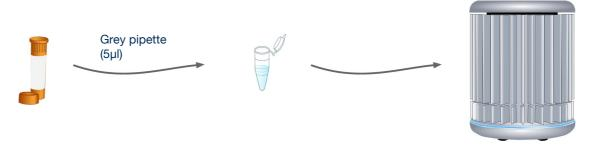
For every reaction to be run, use the grey pipette to add 5µl of your Mumps primers/probe mix to every tube.
