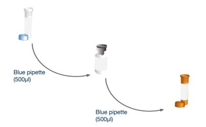
Use the blue pipette to transfer 500µl\* of the oasig Master Mix resuspension buffer into the tube of lyophilised oasig Master Mix and mix well by gently swirling. Then transfer all of that master mix into the brown tube labelled L.acidophilus primers/probe.
