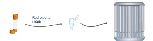
For every reaction to be run, use the red pipette to add  $10\mu$ l of your L.acidophilus reaction mix to every tube.
