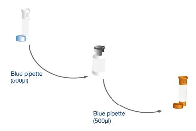
Use the blue pipette to transfer 500µl\* of the oasig Master Mix resuspension buffer into the tube of lyophilised oasig Master Mix and mix well by gently swirling. Then transfer all of that master mix into the brown tube labelled P.theridion primers/probe.
