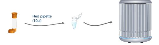
For every reaction to be run, use the red pipette to add 10µl of your P.theridion reaction mix to every tube.
