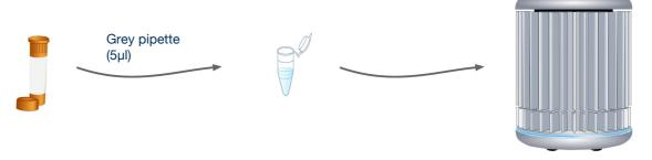
For every reaction to be run, use the grey pipette to add 5µl of your Betanodavirus primers/probe mix to every tube.
