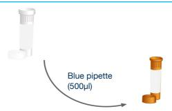
Then use the blue pipette to transfer 500µl of water into the brown tube labelled Betanodavirus primers/probe. Cap and shake tube to mix. A thorough shake is essential to ensure that all components are resuspended. Failure to mix well can produce poor kit performance.
