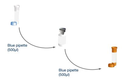
Use the blue pipette to transfer 500µl\* of the oasig Master Mix resuspension buffer into the tube of lyophilised oasig Master Mix and mix well by gently swirling. Then transfer all of that master mix into the brown tube labelled S.subterranea primers/probe.
