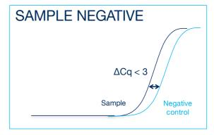
If the sample amplifies < 3 Cq earlier than the negative control then the positive sample result is invalidated and a negative call is the correct result.
