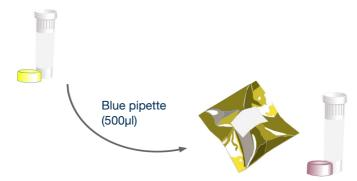
Use the blue pipette to transfer 500µl of template preparation buffer into the positive control template tube. Cap and shake tube to mix.
