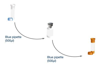
Use the blue pipette to transfer 500µl\* of the oasig Master Mix resuspension buffer into the tube of lyophilised oasig Master Mix and mix well by gently swirling. Then transfer all of that master mix into the brown tube labelled HPV18 primers/probe.
