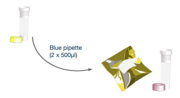
Use the blue pipette to transfer  $1000\mu l$  (2 x  $500\mu l$ ) of template preparation buffer into the positive control template tube. Cap and shake tube to mix.
