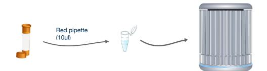
For every reaction to be run, use the red pipette to add 10µl of your V.cholerae\_subsp reaction mix to every tube.
