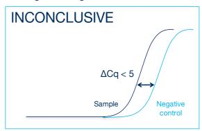
If the sample amplifies < 5 Cq earlier than the negative control then the positive sample result is invalidated and the result should be determined inconclusive due to test contamination. The test for this smaple should be repeated.
