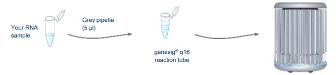
For each sample you wish to analyse, use the grey pipette to add 5  $\mu$ l of your RNA sample to the required reaction tube (already containing primer/probe mix and oasig<sup>®</sup>PLUS OneStep Lyophilised qPCR Master Mix). Close these tubes after adding the sample. Always change pipette tips between samples.
