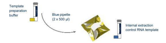
Use the blue pipette to transfer 1000  $\mu$ l (2 x 500  $\mu$ l) of template preparation buffer into the Internal Extraction Control RNA template tube. Cap and shake the tube to mix.
