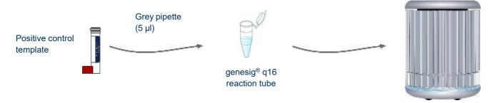
Take great care when setting up your positive control. The positive control template has the potential to give you a false positive signal in your other samples. Set positive controls up last after all other sample tubes are closed. Always change pipette tips between samples. You may even choose to set up positive controls in a separate room.
