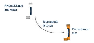
Then use the blue pipette to transfer 500 µl of water into the brown tube labelled HAV primer/probe mix. Cap and leave for 10 minutes to rehydrate. Then shake tube to mix. A thorough shake is essential to ensure that all components are resuspended. Failure to mix well can produce poor kit performance.
