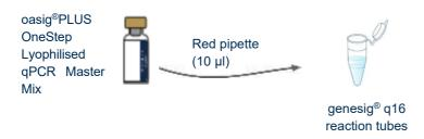
For every reaction to be run, use the red pipette to add 10 µl of the oasig®PLUS OneStep Lyophilised qPCR Master Mix to the reaction tubes containing primer/probe mix.
