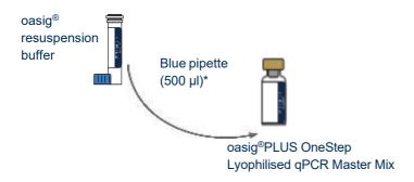
Use the blue pipette to transfer 500 µI\* of the oasig® resuspension buffer into the tube of oasig®PLUS OneStep Lyophilised qPCR Master Mix and mix well by gently swirling.
