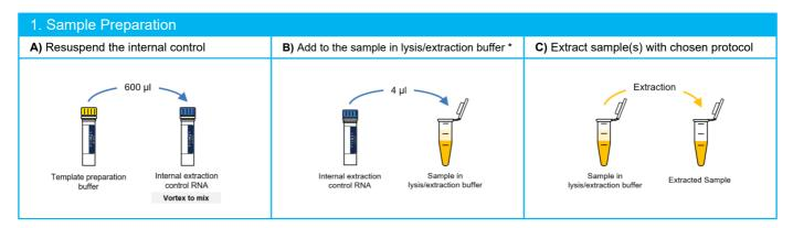
\*NOTE –DO NOT add internal extraction control RNA directly to the unprocessed biological sample as this will lead to degradation and a loss in signal.
