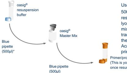
Use the blue pipette to transfer 500µl\* of the oasig® Master Mix resuspension buffer into the tube of lyophilised oasig® Master Mix and mix well by gently swirling. Then transfer all of that master mix into the brown tube labelled Acanthamoeba\_spp\_v2.0 primers/probe.
