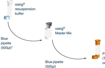
Use the blue pipette to transfer 500µl\* of the oasig® Master Mix resuspension buffer into the tube of lyophilised oasig® Master Mix and mix well by gently swirling. Then transfer all of that master mix into the brown tube labelled C.difficile toxB v2.0 primers/probe.
