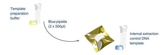
Use the blue pipette to transfer  $1000\mu I$  (2 x  $500\mu I$ ) of template preparation buffer into the Internal Extraction Control DNA template tube. Cap and shake tube to mix.
