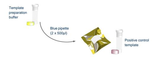
Use the blue pipette to transfer  $1000\mu I$  (2 x  $500\mu I$ ) of template preparation buffer into the positive control template tube. Cap and shake tube to mix.
