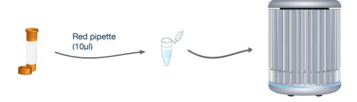
For every reaction to be run, use the red pipette to add 10µl of your ETEC reaction mix to every tube.
