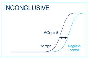
If the sample amplifies < 5 Cq earlier than the negative control then the positive sample result is invalidated and the result should be determined inconclusive due to test contamination. The test for this smaple should be repeated.
