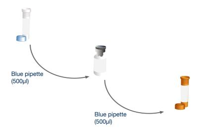
Use the blue pipette to transfer 500µl\* of the oasig Master Mix resuspension buffer into the tube of lyophilised oasig Master Mix and mix well by gently swirling. Then transfer all of that master mix into the brown tube labelled EHV-5 primers/probe.
