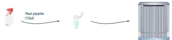
For every reaction to be run, use the red pipette to add 10µl of the oasig OneStep Master Mix to the tubes containing primer/probe mix.
