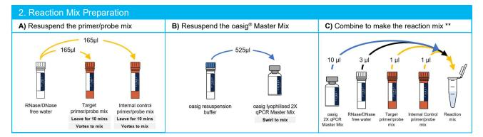
\*NOTE – Displayed amounts are required for each reaction. Multiply each volume by the number of reactions required including overage.
