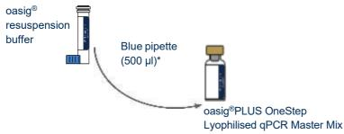
Use the blue pipette to transfer 500 µI\* of the oasig® resuspension buffer into the tube of oasig®PLUS OneStep Lyophilised qPCR Master Mix and mix well by gently swirling.
