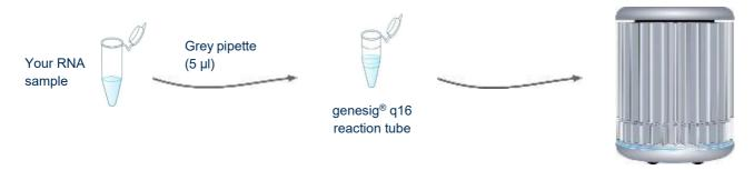
For each sample you wish to analyse, use the grey pipette to add 5 µl of your RNA sample to the required reaction tube (already containing primer/probe mix and oasig<sup>®</sup>PLUS OneStep Lyophilised qPCR Master Mix). Close these tubes after adding the sample. Always change pipette tips between samples.
