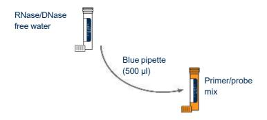
Then use the blue pipette to transfer 500 µl of water into the brown tube labelled HCV v2.0 primer/probe mix. Cap and leave for 10 minutes to rehydrate. Then shake tube to mix. A thorough shake is essential to ensure that all components are resuspended. Failure to mix well can produce poor kit performance.
