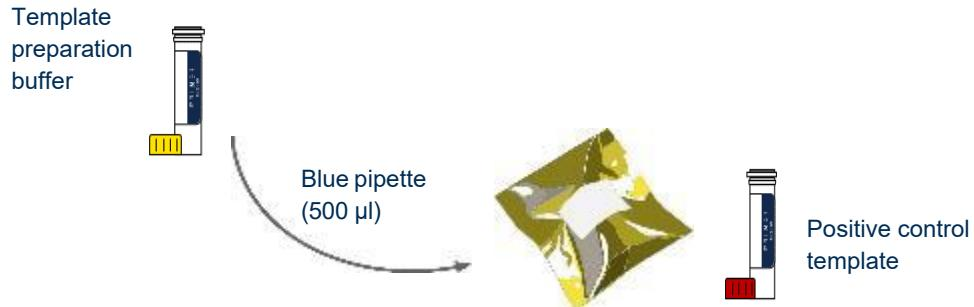
Use the blue pipette to transfer 500 µl of template preparation buffer into the positive control template tube. Cap and shake tube to mix.
