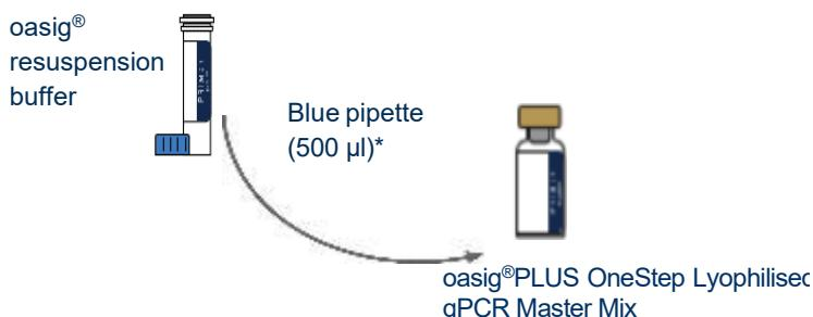
Use the blue pipette to transfer 500 µl\* of the oasig® resuspension buffer into the tube of oasig®PLUS OneStep Lyophilised qPCR Master Mix and mix well by gently swirling.
