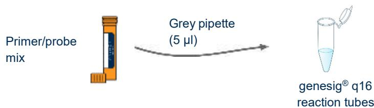
For every reaction to be run, use the grey pipette to add 5 µl of your H5 v2.0 primer/probe mix to every genesig® q16 reaction tube.
