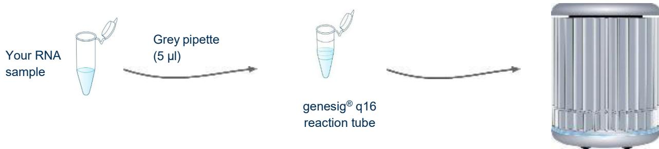
For each sample you wish to analyse, use the grey pipette to add 5 µl of your RNA sample to the required reaction tube (already containing primer/probe mix and oasig®PLUS OneStep Lyophilised qPCR Master Mix). Close these tubes after adding the sample. Always change pipette tips between samples.
