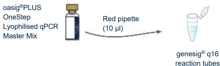
For every reaction to be run, use the red pipette to add 10 µl of the oasig®PLUS OneStep Lyophilised qPCR Master Mix to the reaction tubes containing primer/probe mix.
