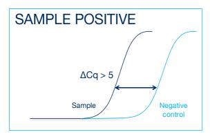
If the sample amplifies > 5 Cq earlier than the negative control then the sample should be reinterpreted (via the table above) with the negative control verified as negative.
