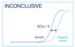
If the sample amplifies < 5 Cq earlier than the negative control then the positive sample result is invalidated and the result should be determined inconclusive due to test contamination. The test for this sample should be repeated.
