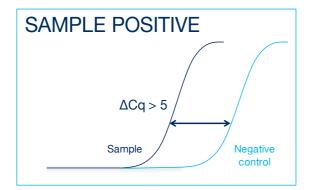
If the sample amplifies > 5 Cq earlier than the negative control then the sample should be reinterpreted (via the table above) with the negative control verified as negative.
