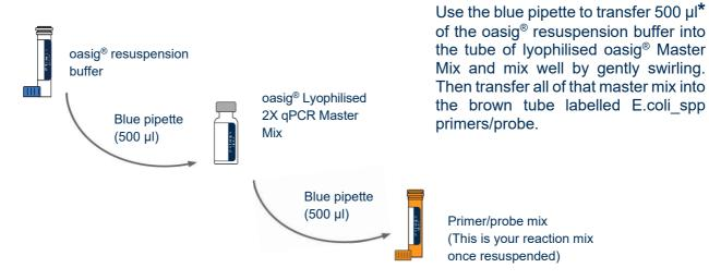
\*Transferring 525  $\mu$ I of the oasig® resuspension buffer to your oasig® Lyophilised 2X qPCR Master Mix (instead of the 500  $\mu$ I recommended above) will enable you to take full advantage of the 50 reactions by accounting for volume losses during pipetting. In order to do so with the genesig® Easy fixed volume pipettes use 1x blue, 2x red and 1x grey pipettes to make the total volume. Please be assured that this will not adversely affect the efficiency of the test.
