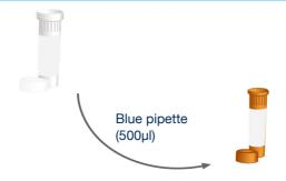
Then use the blue pipette to transfer 500µl of water into the brown tube labelled BLV v1.1 primers/probe. Cap and shake tube to mix. A thorough shake is essential to ensure that all components are resuspended. Failure to mix well can produce poor kit performance.
