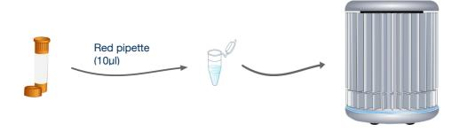
For every reaction to be run, use the red pipette to add 10µl of your C.abortus reaction mix to every tube.
