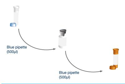
Use the blue pipette to transfer 500µl\* of the oasig Master Mix resuspension buffer into the tube of lyophilised oasig Master Mix and mix well by gently swirling. Then transfer all of that master mix into the brown tube labelled C.fetus-venerialis primers/probe.
