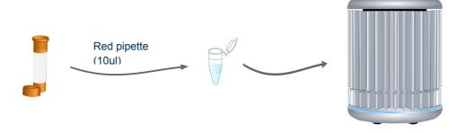
For every reaction to be run, use the red pipette to add 10µl of your C.psittaci reaction mix to every tube.
