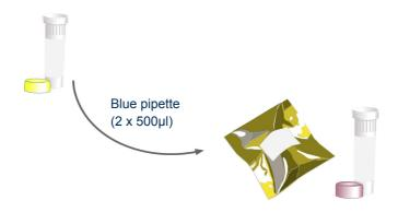
Use the blue pipette to transfer  $1000\mu$ I (2 x  $500\mu$ I) of template preparation buffer into the positive control template tube. Cap and shake tube to mix.
